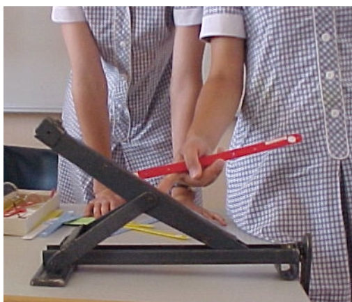
Figure 5. Students D and E: exploring the operation of the triangular linkage car jack.
